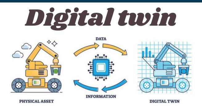
Digital twin is a virtual representation of an object or system designed to reflect a physical object accurately. It spans the object's lifecycle, is updated from real-time data and uses simulation, machine learning and reasoning to help make decisions.
