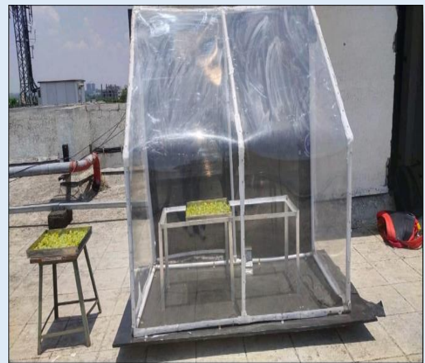
Fig:- Greenhouse Based Solar Dryer
