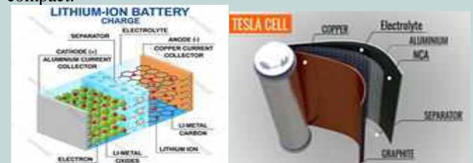
A standard Tesla cell has a voltage between 3 and 4.2 volts. Many such Tesla cells are connected in series and a parallel fashion to form a module. 16 such modules are connected in series to form a battery pack in a Tesla car.
