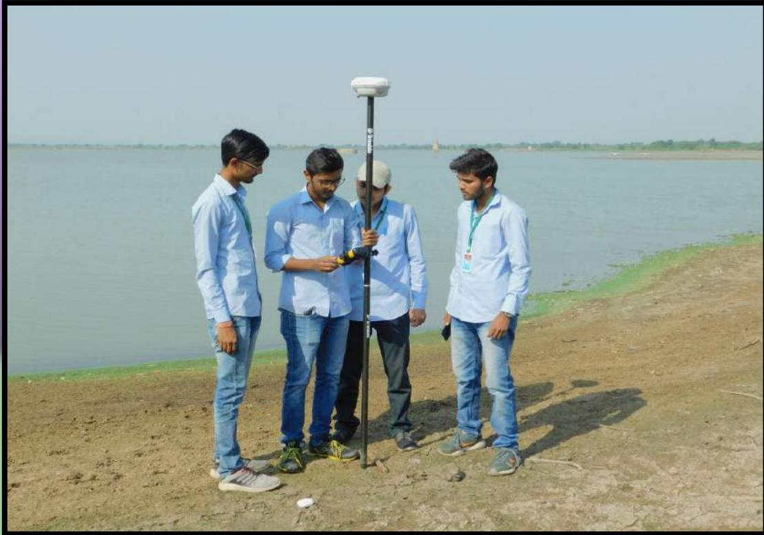
Taking readings at various points using DGPS Rover
