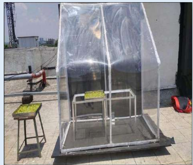
Fig:- Greenhouse Based Solar Dryer
