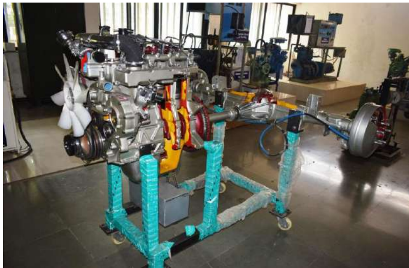
Fig. 2 Photograph of motorised cut section of internal combustion engine
